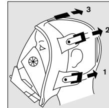
**Leak test:** Seal the mask connector and breathe in to produce a negative pressure. Hold your breath for a moment. The negative pressure should be maintained. If not, retighten the straps. Repeat the leak test twice. **Never use a full-face mask that leaks!**
