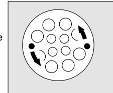
**Replace exhalation valve disc:** Refer to "Visual inspection of exhalation valve". Fit protective cap so that it engages.
