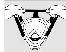
Fit harness over the head, pulling back until the head strap fits smoothly. Adjust full-face mask until it fits properly.
